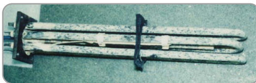
June 15, 1997 [Before Installation] Scale is stuck firmly all over.
