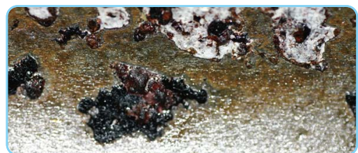
Calcium Covering underneath Iron Rust Layer Rust Layer Bottom and Bare Metal
