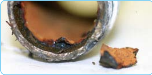
Pipe wall has black rust after installing BW
